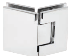
Cat. No. JRG045XX 135° Glass-to-Glass (factory set for 5° tighter closure into shower interior)
